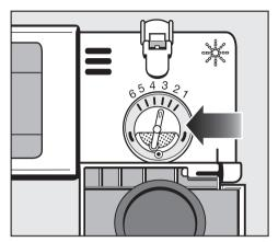
The dosage selector is preset to 3. This dispenses approximately 3 ml of rinse aid per program. It can be adjusted from 1 to 6.
